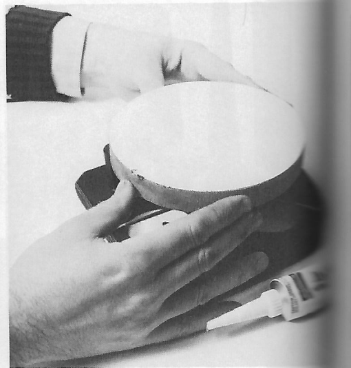
Step 2: Lower the mirror onto three adhesive blobs; 16d nails act as spacers.
