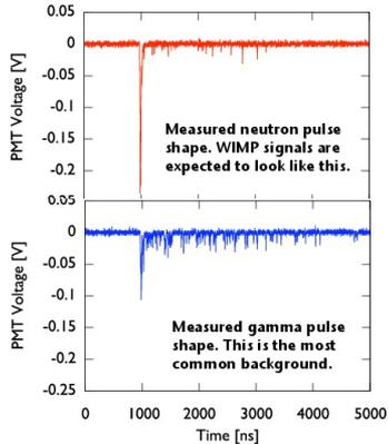
FIGURE 2: Neutron and gamma pulse shapes.
