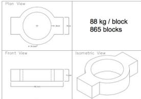
Geometry of the lead blocks for HALO-I
