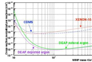
FIGURE 12: Expected Dark Matter sensitivities for a 1000 kg liquid argon detector with a 20 keVee threshold (purple) and a 19 keVee threshold (green) for argon depleted in  $^{39}\text{Ar}$  by a factor of 20. The current sensitivities of the CDMS and XENON detectors are shown for comparison.
