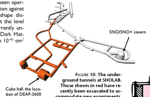
FIGURE 10: The underground tunnels at SNOLAB. Those shown in red have recently been excavated to accommodate new experiments.
