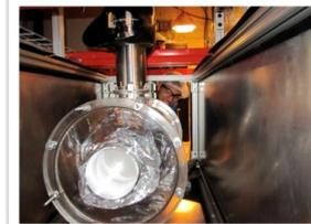
FIGURE 6: View of the DEAP-1 detector without the PMTs installed.
