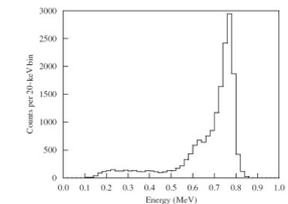
Fig. 1. NCD array neutron-capture spectrum from a uniformly distributed <sup>238</sup>Na calibration. The peak at 764 keV corresponds to deposition of the full kinetic energy of the proton and triton in the active volume of the NCD. The 573-keV shoulder, caused by total absorption of the triton's energy in the wall, is distorted by space-charge effects, discussed in Section 6.1. The 191-keV shoulder is caused by total absorption of the proton's energy in the wall.
