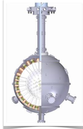
FIGURE 7: 3D rendering of the DEAP-3600 detector showing the acrylic vessel, light guides, PMTs and shell.
