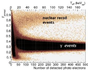
FIGURE 3:  $F_{prompt}$  vs. Energy for events from an AmBe source.
