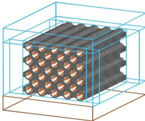
The lead blocks will be arranged into 32 horizontal stacked columns 3 m long. Four 3 m long <sup>3</sup>He counters will be placed into each column of lead (shown in orange). Some neutron moderator, polyethylene, (shown in white) increases capture efficiency.
