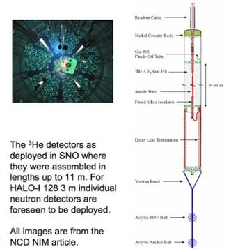
The <sup>3</sup>He detectors as deployed in SNO where they were assembled in lengths up to 11 m. For HALO-I 128 3 m individual neutron detectors are foreseen to be deployed.
