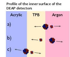
FIGURE 11: Possible backgrounds from the inner detector surface.
